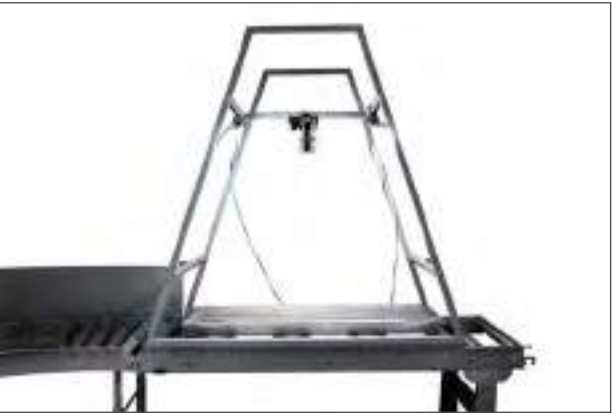
Roller racking camera frame fixed
